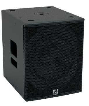
The X115 is a very compact subwoofer designed to augment the low frequency performance of BlacklineX Series full-range systems. It comprises a long excursion 15" (380mm)/3" (75mm) voice coil driver in a bass reflex enclosure and can be used singly, stacked or flown via integral M10 inserts. Four large ports contribute to a reduction in air noise at high output levels.
