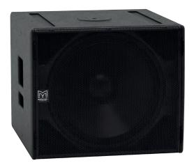
The SX118 is a compact, high performance subwoofer that extends the low frequency operating range of the system to 47Hz and provides exceptional low frequency output for such a compact enclosure. An ideal partner for the WPM, it features a long-excursion 18" (460mm)/4" (100 mm) voice coil driver with a water-resistant cone and triple roll surround in a compact reflex enclosure.
