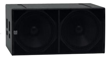
The SX218 achieves the ultimate in subwoofer performance for the most demanding applications – delivering very high output levels and superb transient performance with minimal distortion it is the perfect partner to WPC, with one subwoofer to every 2 top boxes required. With an operating range of 35Hz-150Hz  $\pm$  3dB, it houses dual 18" long-excursion (460mm)/4" (100mm) voice coil drivers with water-resistant cones and triple roll surrounds. Each driver is rated to handle 1000 watts
