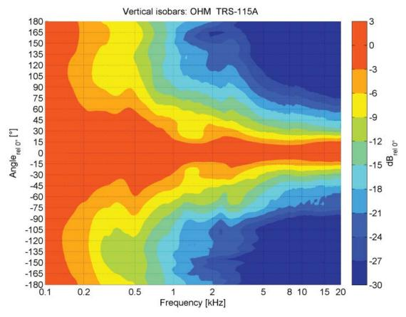
All Measurements are executed by the IFAA Institute for Acoustics in Aachen, Germany measurement conditions 4PI environment for full range cabinets, 2Pi environment for subwoofers.
