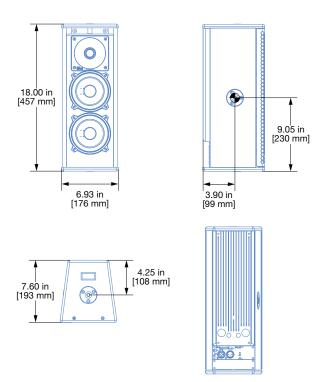
The UPM-1P is a remarkably compact, self-powered, professional sound reinforcement loudspeaker system. It is ideally suited to applications requiring a relatively small and inconspicuous loudspeaker that can also provide high sound pressure levels, extremely low distortion, and uniform directional control.
